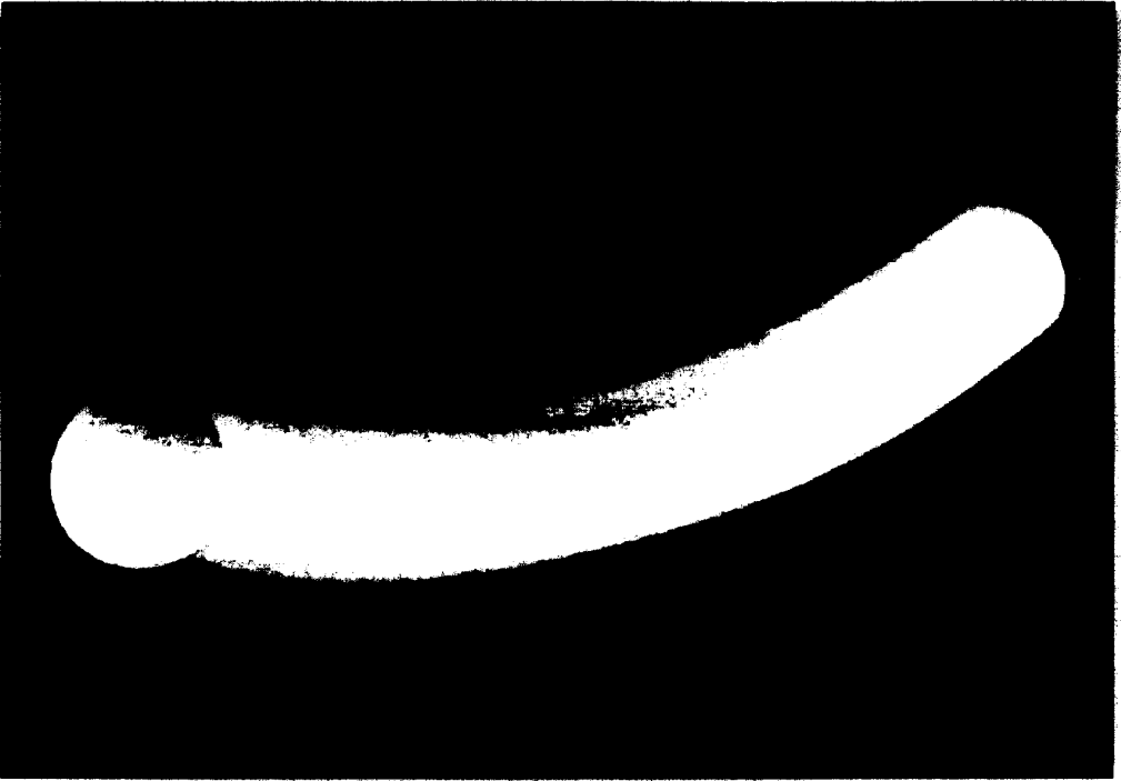
Fig. 18. Graphical reproduction of calculated deformed shell configuration illustrating localization ( D/t = 19.5 ).
